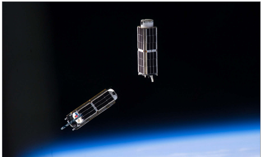
Figure 3 | A set of NanoRacks' CubeSats as photographed by an Expedition 38 crew member aboard the International Space Station. The CubeSats program contains a variety of experiments, including Earth observations and advanced electronics testing. Photo courtesy of NASA.
